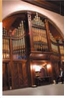
Dating from 1861 this rare concert organ is still in use today and provides a magnificent backdrop to the stage of the Albert Hall. It is operated by water which drives a pump compressing air into bellows, which in turn blows the organ pipes as the keys are played. It was moved to the Albert Hall in 1891.
